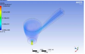
Figure.10 Velocity distribution for 100 mm Outlet diameter
