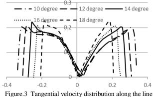
Figure.3 Tangential velocity distribution along the line drawn at 0.1 meters form bottom face for different cone angle.
