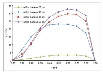
Tangential velocity distribution for different orifice diameters [1]
