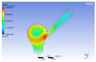
Figure.9 Velocity distribution for500mm Outlet diameter
