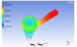
Figure. 8 Pressure distribution for 400 mm outlet diameter
