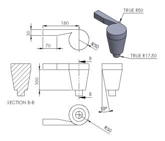
Figure.1 Dimensions of the basin and runner
