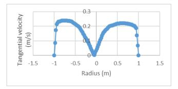
Tangential velocity for 300 mm outlet diameter from analysis.
