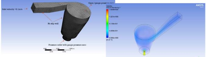
Figure.7 Meshed model with boundary conditions **Pressure distribution**
